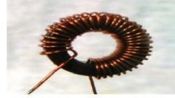
Ferrite core Toroidal transformer
